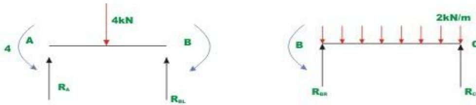
**Fig.13.2 (c) Free - body diagram of two members**
